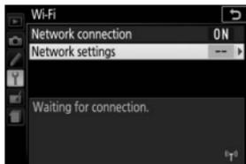
Highlight **Push-button WPS** and press **▶** to ready the camera for a WPS connection. The camera will wait about two minutes for a WPS connection request from the smart device. To extend the wait time, press **OK**.
