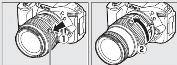
*Retractable lens barrel button*
