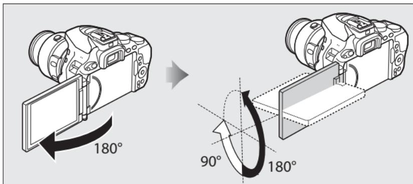
**Normal use:** Fold the monitor against the camera face out. The monitor is normally used in this position.
